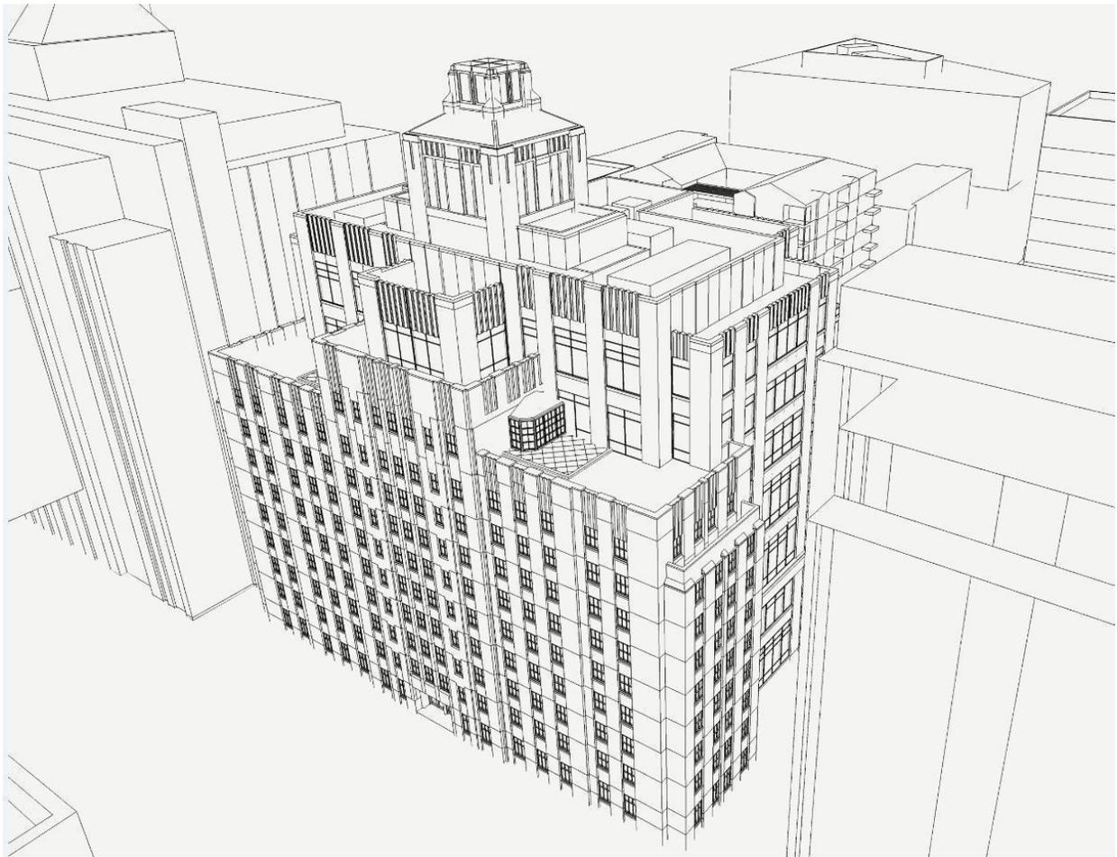
Along the Terry Avenue eastern façade, the new Harborview Hall Adaptive reuse section eastern façade would be visible. *See Figure 10.* The eastern façade materials would include plain and patterned brick veneer, spandrel glass, metal panel wall, glass and terra cotta caps.
